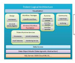
Figure 1: Diagram of the Trident logical architecture
