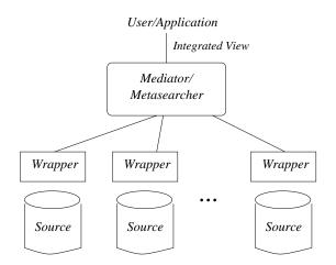
Figure 1: Both metasearchers and mediators use wrappers around the underlying databases. These wrappers provide a relatively uniform view of these databases.
