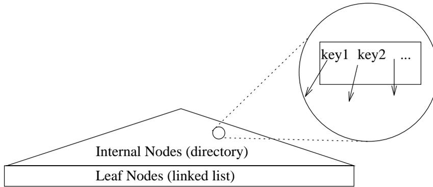
Figure 5: Sketch of a database index tree.
